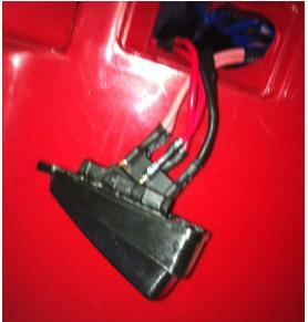
3. Pls make sure the forward and reverse switch is plugged firmly.
