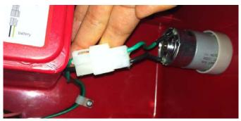
2. Turn the vehicle body to check if the pedal switch is connected to the wiring firmly.
