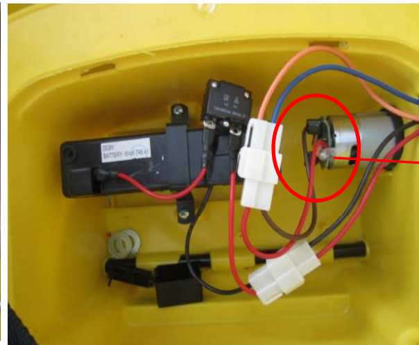
3. The cables connections for pedal switch
