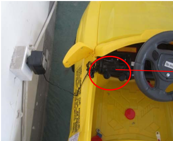
5. Connect the wire to the battery (positive terminal)
