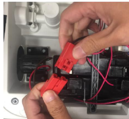
STEP 5 (Gearbox cable)
