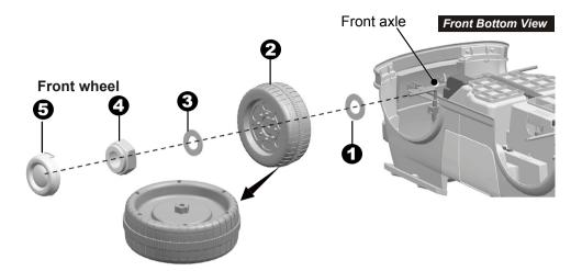
Remove all the parts from the front axle.
