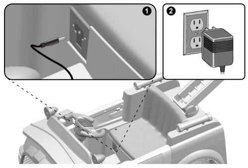
1. Plug the charger port into the input socket. (the socket is below the seat)
